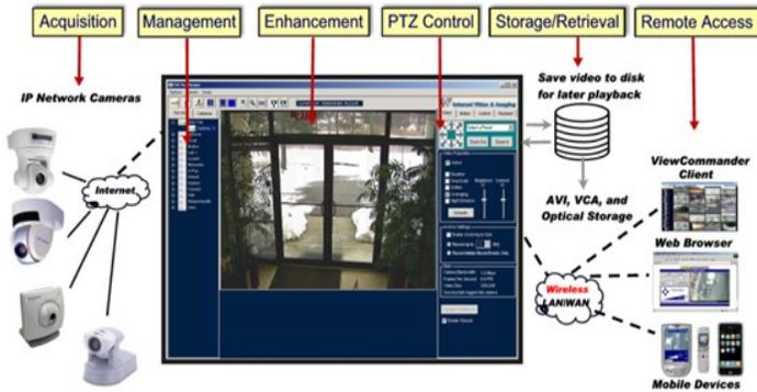
**ViewCommander-NVR** connects to a wide variety of IP cameras which can be located anywhere on the Internet. Through ViewCommander, you can view and control Pan/Tilt/Zoom (PTZ) features for each camera.
